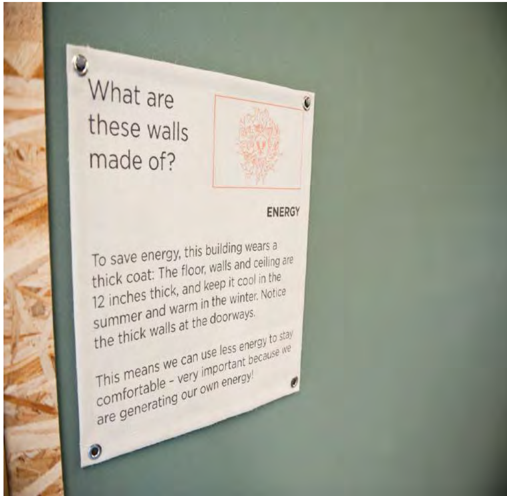
Figure 8: What are these walls made of? SIPs
